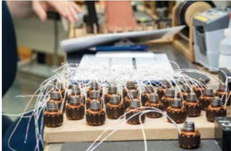
A batch of motor windings ready for final assembly.
