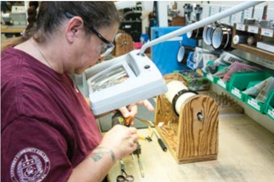
Operator preparing subassembly for motor windings.
