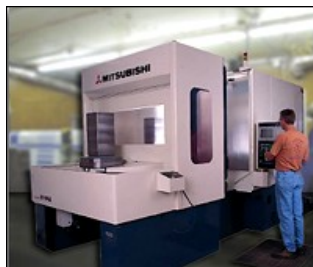
A two pallet Mitsubishi Horizontal CNC Machining Cen-
