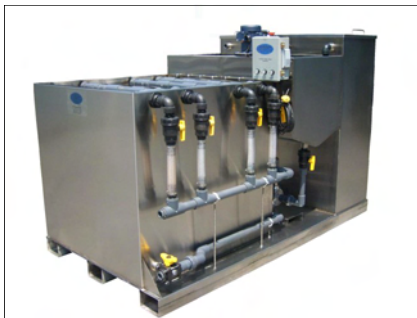
An EV4BF (Everclean 4 Bag Filters). This machine separates out suspended solids, emulsified oils and heavy metals. It encapsulates the contaminants and produces a non-leachable sludge that will meet TCLP and is non-hazardous.
