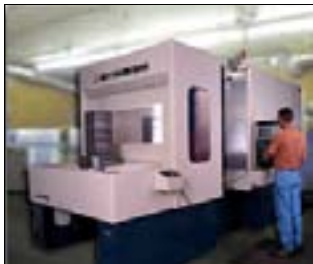
A two pallet Mitsubishi Horizontal CNC Machining Center.
