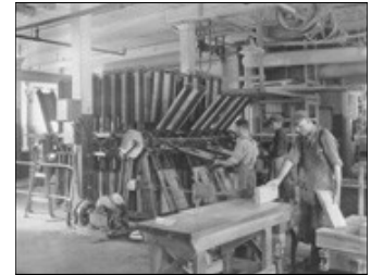
A Taylor Clamp Carrier from the 1920's. James L. Taylor Manufacturing Co. has been a member of the Council of Industry since 1912 and is this month's member profile.
