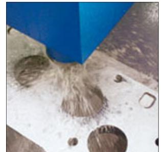
One of Blaser Swisslube's products, Blasocut, in action. Blasocut is used in the machining and grinding of ferrous and non-ferrous materials.
