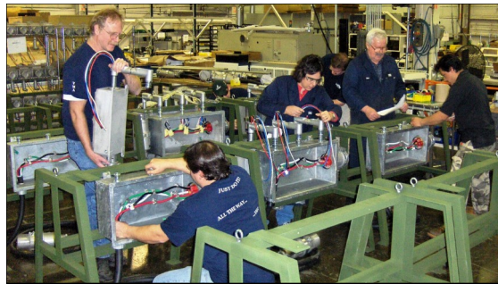
VMA's skilled technicians team together to build power distribution assemblies.
