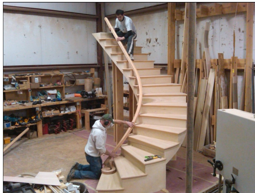
This photo shows a curved stair being fitted with a custom bent railing.
