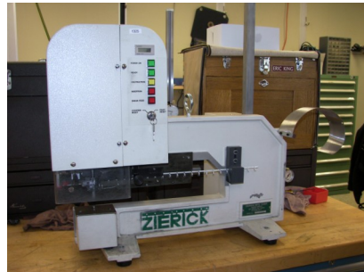
A machine developed by Zierick to install the components they manufacture.
