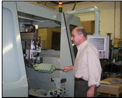
Jim Faulkner removing a completed wax assembly from an APAS machine.
